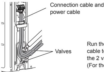
Run the connection cable and power supply cable to the rear of the outdoor unit between the 2 valves as shown in the figure. (For the switch cover to be easily installed.)
