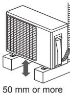
If the unit is installed in a region that is exposed to high winds, freezing conditions, freezing rain, snow fall or heavy snow accumulation, take appropriate measures to protect it from those elements. To ensure stable operation, the outdoor unit must be installed on a raised stand or rack, at or above the anticipated snow depth for the region. The installation of snow hoods and drift prevention fencing is recommended when blowing and drifting snow is common to the region.
