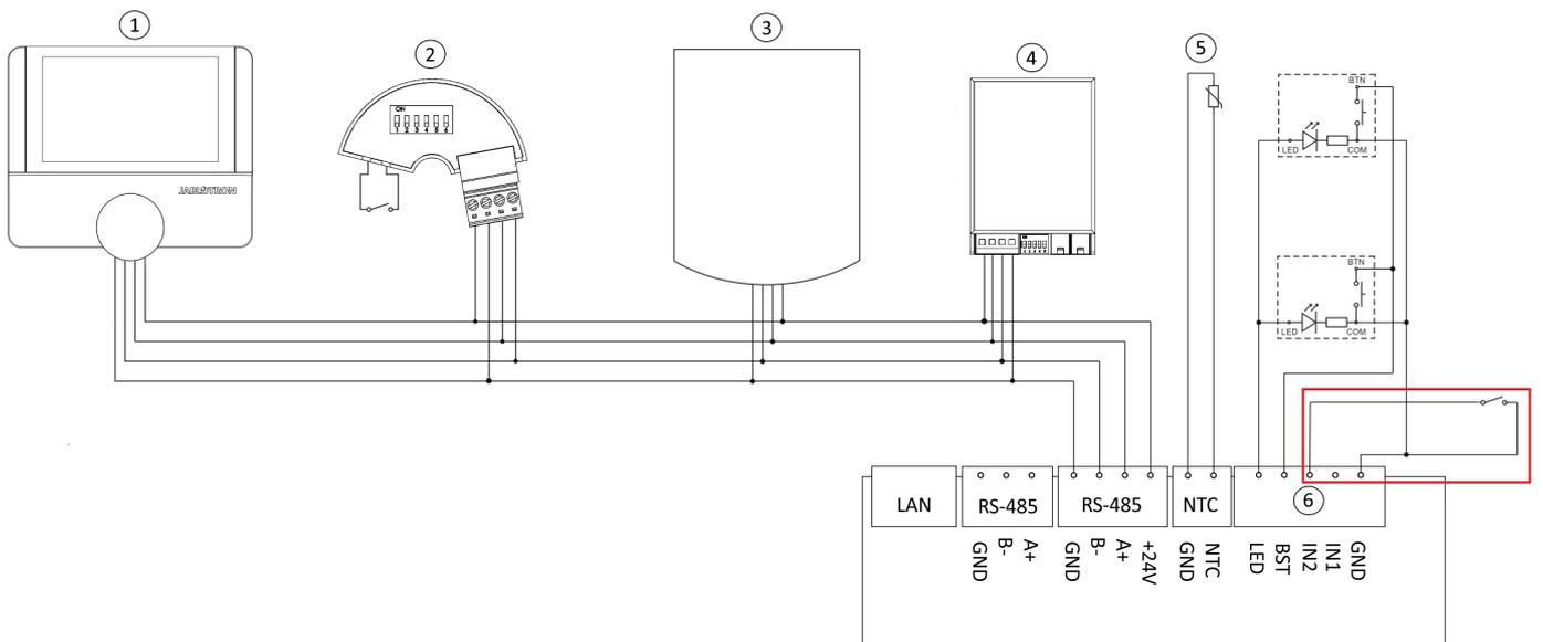
Example of analog input connection for \*boost, overpressure, circulation\*.
