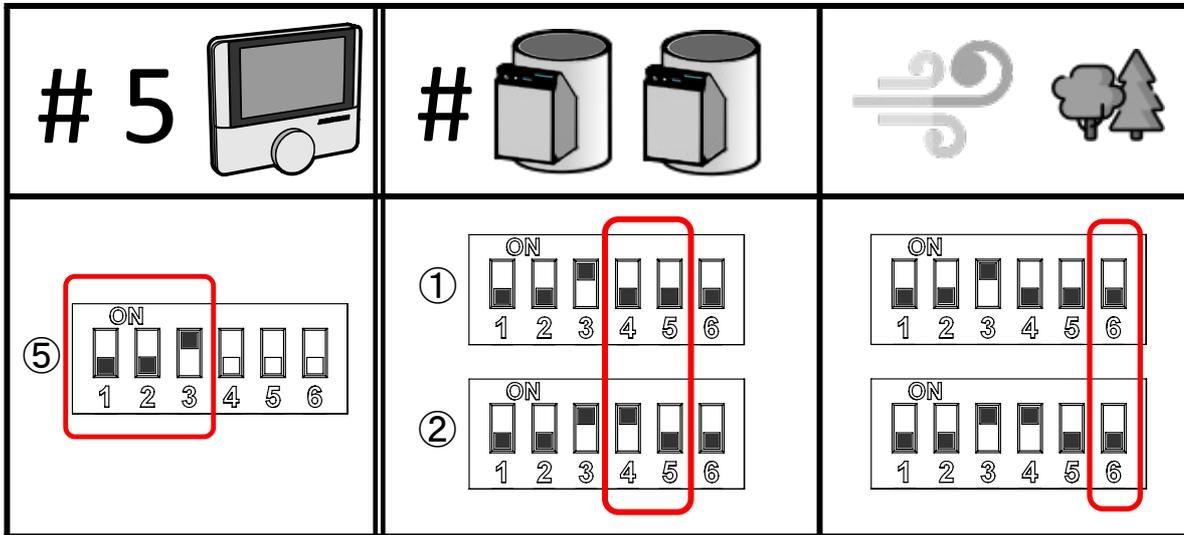
Figure 25 – Example of configuring a supply zone: zone no. 5, two valves, supply
