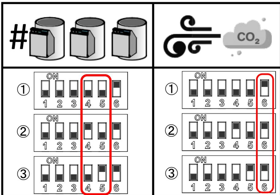
Figure 26 – Example of configuring an extract zone: zone one, three valves, extract
