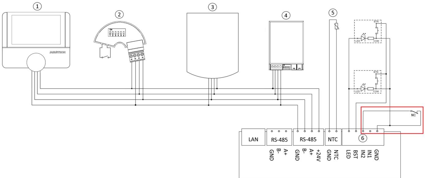
Example of analog input connection for \*emergency shutdown\*.
