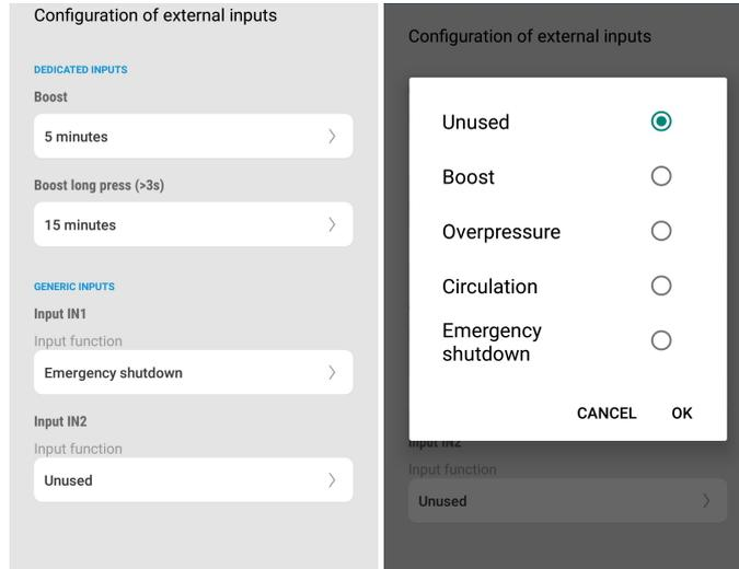
Figure 33 and 34 – Setting the input for emergency shutdown
