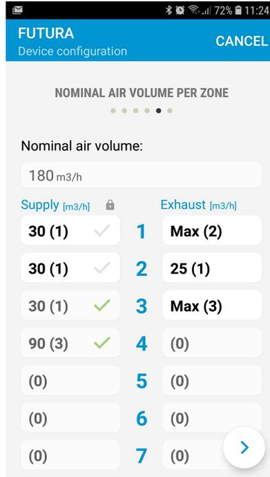
Figure 16 – Setting the nominal airflow of a zone
