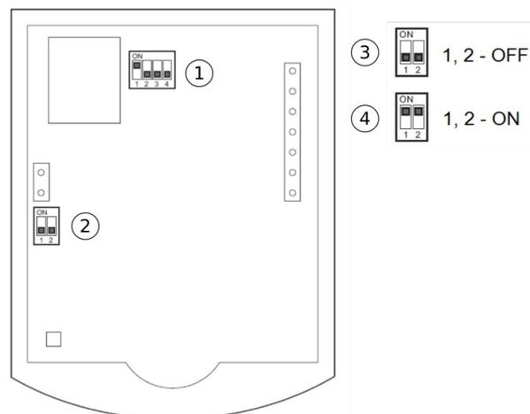
Make sure to always activate (via DIP switch) a terminating resistor to the last device (control panel or sensor) in the line! Always activate the resistor on one device only! The second terminating resistor is connected to Futura.
