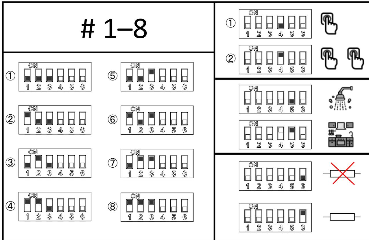
Figure 24 - Setting a button DIP switch
