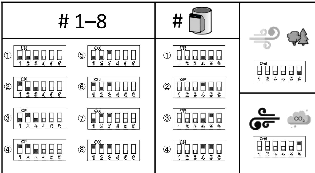
Figure 23 - Setting a valve DIP switch
