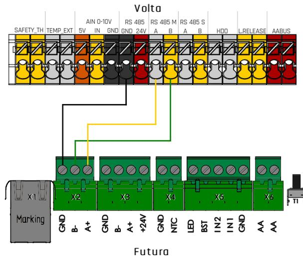
Figure 31 - Volta RS-485 connection
