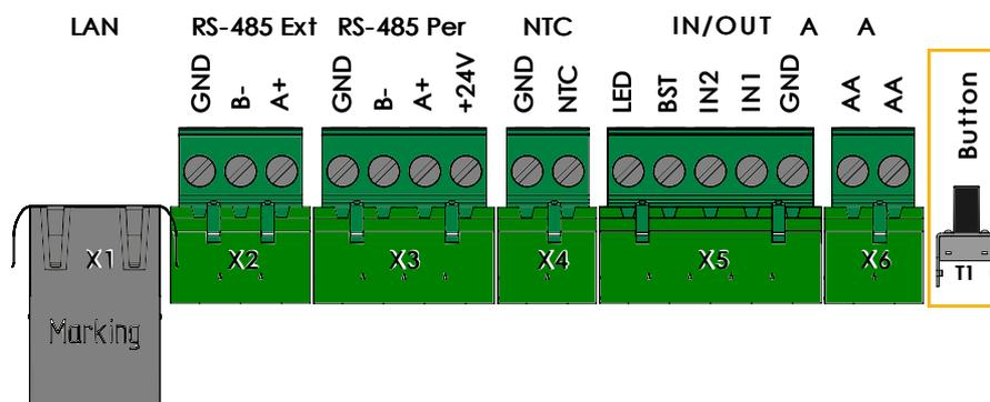
Figure 37 – Filter initialization - hold for 15 seconds, then release
