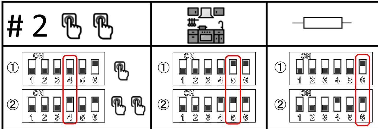
Figure 27 – Example of a button configuration: two buttons, **switch** mode, terminating resistor enabled
