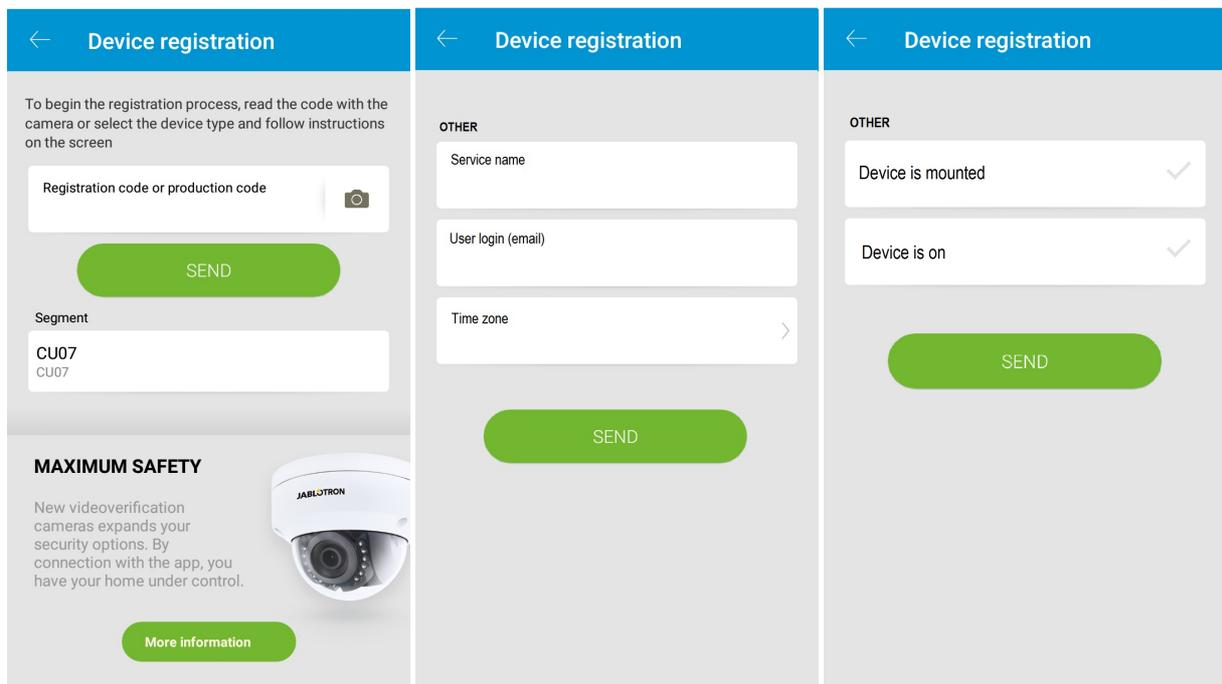
Figure 18 - Entering registration key, Figure 19 - Registration of the device, Figure 20 - Confirmation of other parameters
