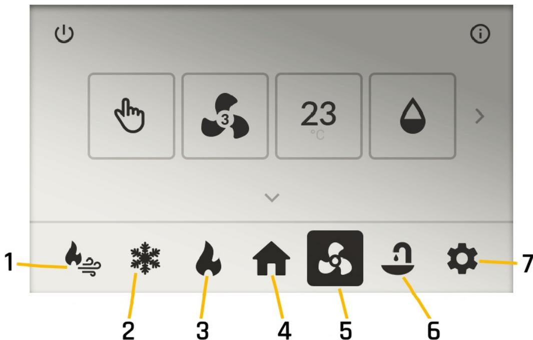
Figure 7 – Quick access tab icons - active ventilation
