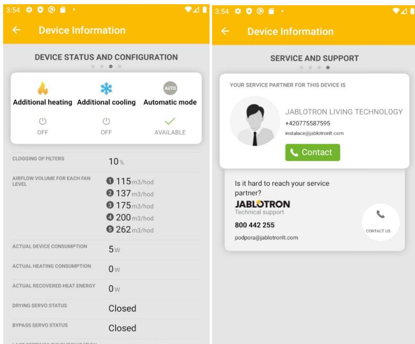
Figure 24 – Flow rates of different ventilation levels, consumption and actuator status, Figure 25 – Your service technician and customer support
