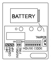
**Note**: More sensors can be connected to each transmitter input (serial combination of N.C. contacts or parallel combination of N.O. contacts). Only dry contacts can be connected to the input terminals of JA-50T transmitter. No external voltage can be connected to these terminals.
